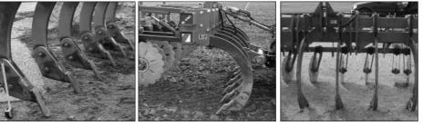
Fig. 1: Front subsoiler with rigid tines and disc coulters
