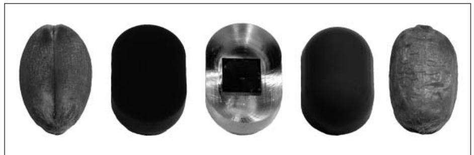
Fig. 1: Grain dummies compared to wheat kernels
