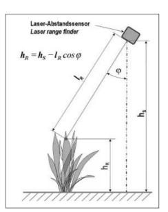
Fig. 2: Calculation of reflection height;  $h_R$  reflection height,  $h_S$  height of sensor,  $I_R$  reflection distance
