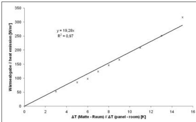
Fig. 3: In the climate chamber experiment heat emission was clearly a function of the temperature difference between the heating mat and room temperature
