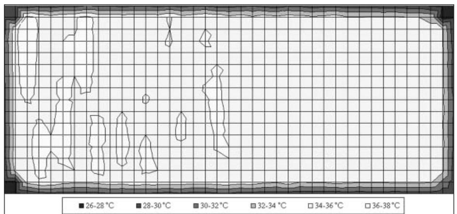
Fig. 2: Heat distribution on the surface of the warm water mat, with the water entering at the top left and leaving at the bottom right (to the next element or back to heater)
