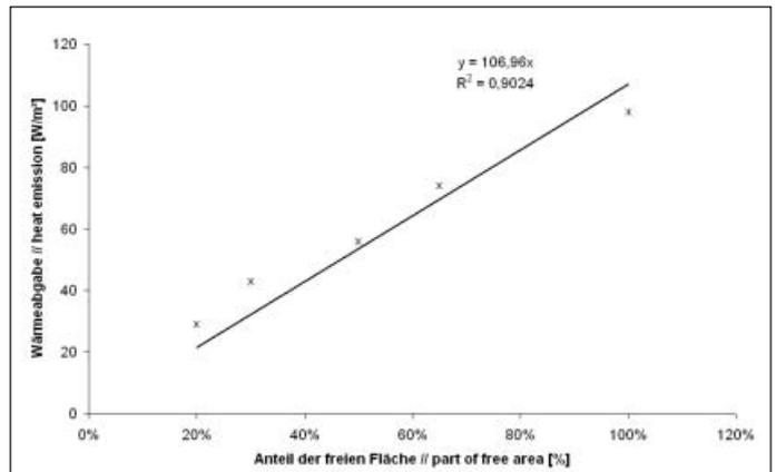
Fig. 4: Heat emission as a function of the free convective area/ the degree of coverage by resting animals (at a temperature difference of 6 Kelvin)
