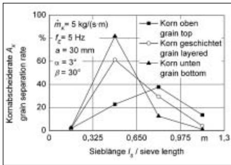
Fig. 3: Influence of layering on the grain separation rate
