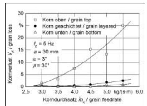
Fig. 2: Influence of layering on the grain loss
