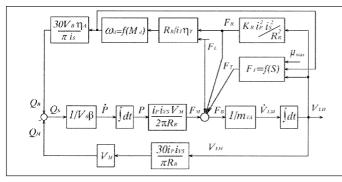
Fig. 3: Block diagram for controlling the auxiliary drive
