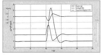
Fig. 4: Result of a simulation calculation: jump from  $\mu_{max}$  = 0.8 to  $\mu_{max}$  = 0.5
