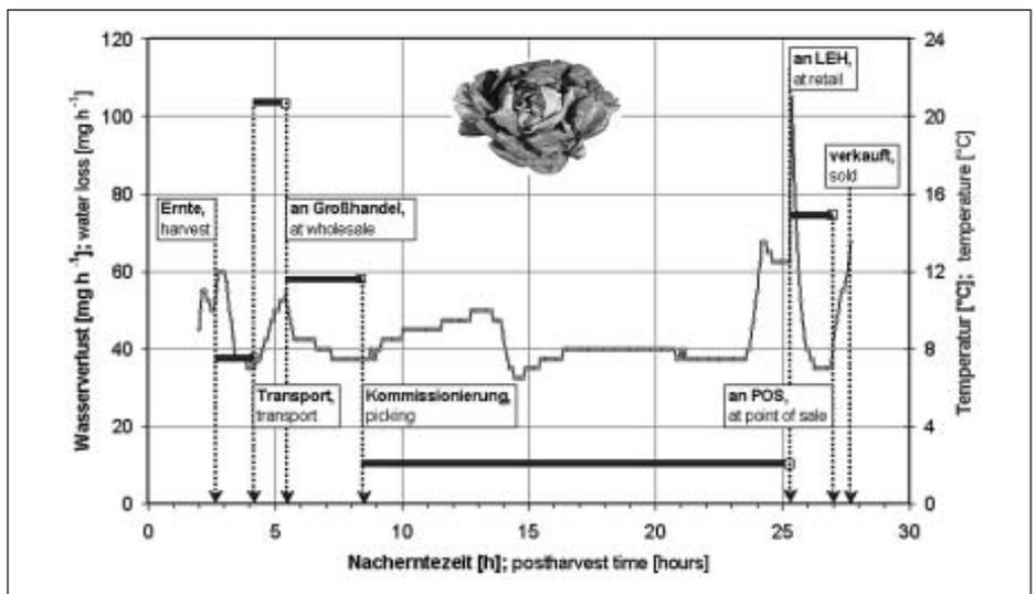
Fig. 2: Control of the climatic loads of lettuce in the postharvest chain by means of temperature devices and evaporation spheres
