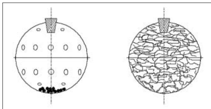
Fig. 1: Scheme of an evaporation sphere with waterholding material (right: dry; left: wetted)
