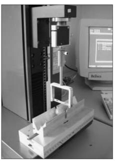
Fig. 1: For cutting, a microtome blade (Feather S35, 0.26 mm thickness), adapted to the universal testing machine (Zwicki 1120, Zwick GmbH & Co. KG, Germany) was used.
