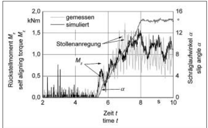
Fig. 2: Self-aligning torque of a pulled wheel at a slip rate angle of  $\alpha' = 0.5/s$ , a static wheel load  $F_z = 20 \text{ kN}$  and  $v_{ix} = 2 \text{ km/h}$
