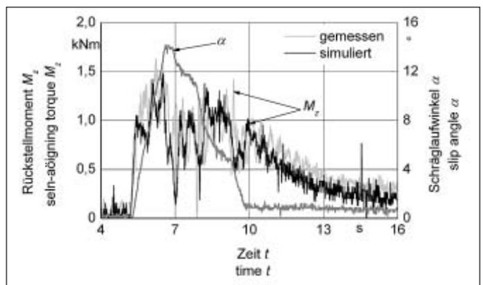
Fig. 4: Self-aligning torque of a pulled wheel during a sign change of the slip rate angle at a wheel load of  $F_z = 20 \text{ kN}$  and  $v_{ix} = 2 \text{ km/h}$
