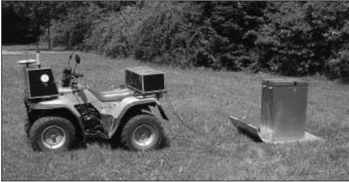
Fig. 2: ATV with RTK-GPS and camera chassis for the determination of the collection of soil straw coverage
