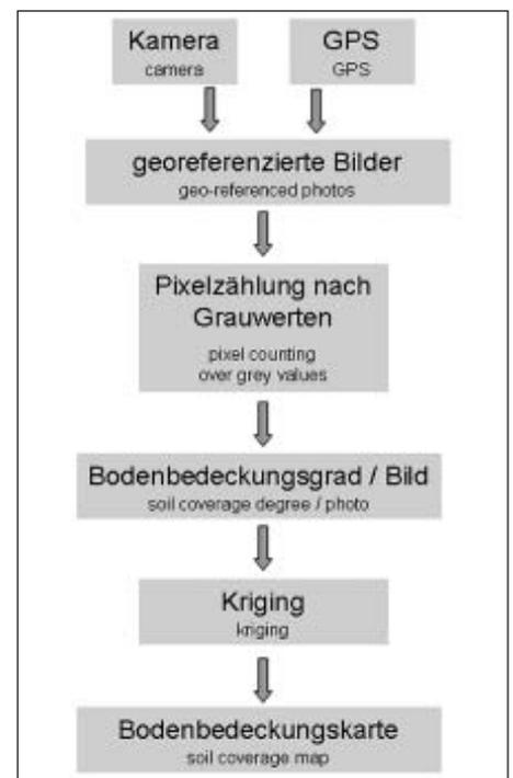
Fig. 4: Procedure for establishing a soil coverage map
