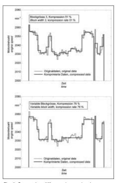
Fig. 2: Comparing different data reduction methods
