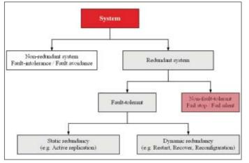
Fig. 2: System redundancy
