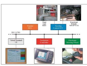
Fig. 3: Schematic network structure of Steer-by-Wire application via ISOBUS
