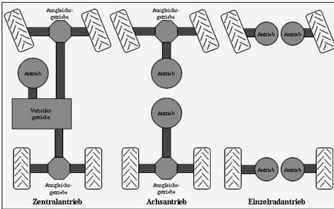
Fig. 2: Schematic configuration of vehicle power trains
