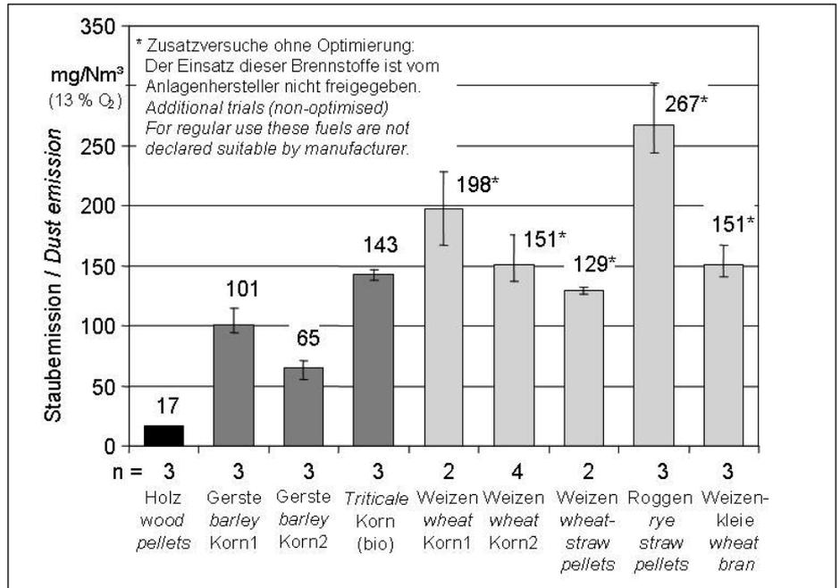
Fig. 3: Total dust emissions using various biofuels (without lime added) in a 30 kW furnace (Guntamatic Powercorn 30) at maximum heat load (n = number of measurements)
