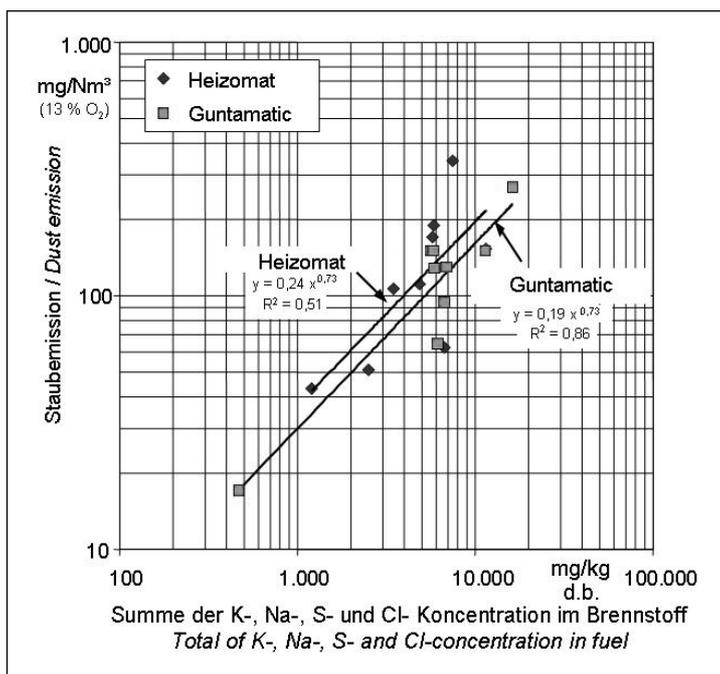
Fig. 2: Total dust emission in the fuels as a function of aerosol forming elements. Regression based on mean values from three to twelve replications per fuel
