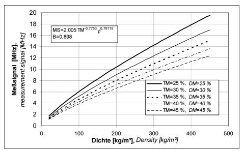
Fig. 1: Effect of the parameters density  $\rho$  and dry matter content DM on the measuring signal MS of a microwave sensor during measuring the density of eleven silage samples (forage maize and gras)
