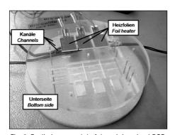
Fig. 2: Preliminary model of the miniaturised PCR unit of the on-chip system
