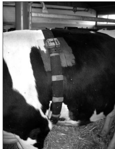
Fig. 1: Belt with two electrodes and heart rate monitor
