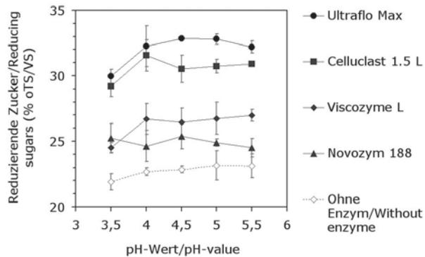
Reducing sugar release after 24 hours of maize straw hydrolysis at different pH values between 3,5 and 5,5; trial in water bath at 50 °C
