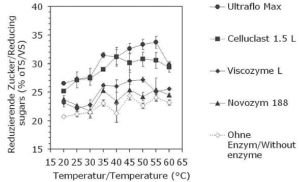
Effect of temperature on reducing sugars content after 24 hours hydrolysis of maize straw at pH 4,5
