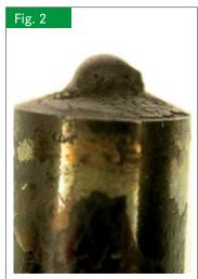
Deposits on the injection nozzle of cylinder 1 of the Fendt Vario 412 after 2653 operating hours
