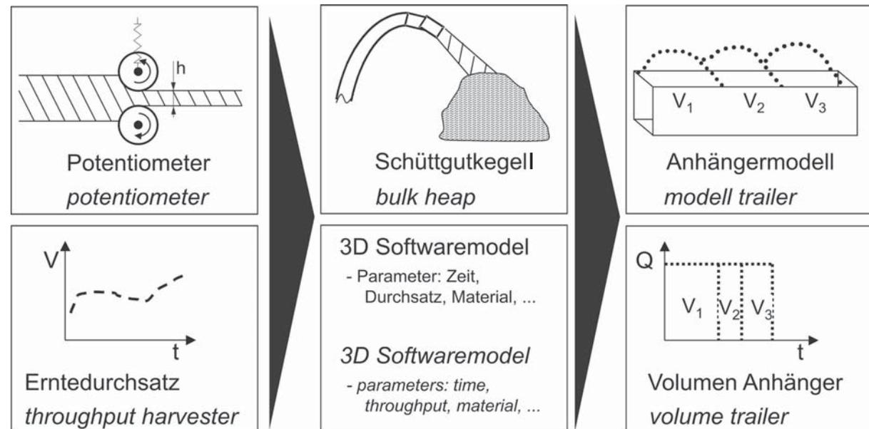
Set up of model based loading of agricultural trailers
