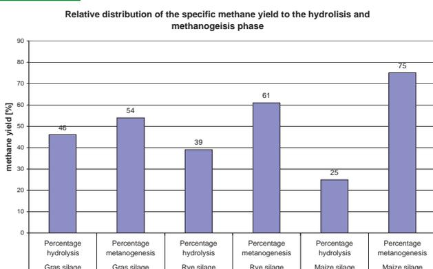
Relative distribution of the specific methane yield of the various stages (hydrolysis and methanogenesis) in the two-phase anaerobic digestion of various renewable resources
