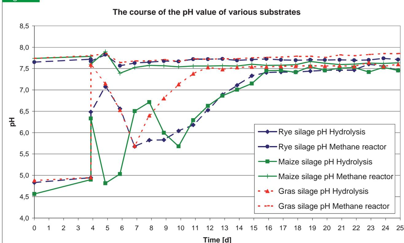
*The development of the pH-values of the substrates grass silage, maize silage and rye silage in a two phase process with a batch hydrolysis*
