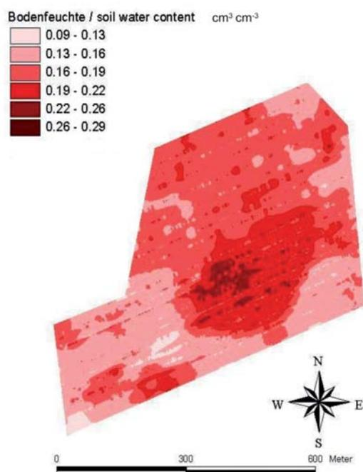
Mapping of the volumetric soil water content in a depth of 10 to 20 cm
