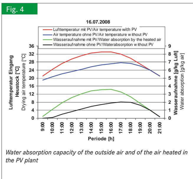
When using the heated air of the photovoltaic plant for drying hay, the drying period can be halved.
