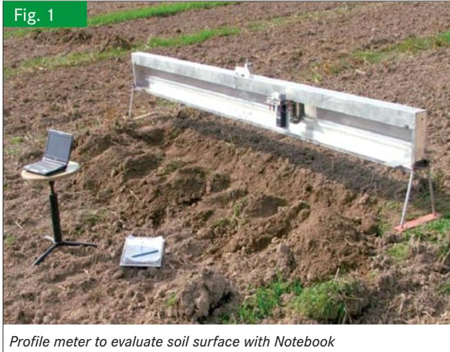
For measuring working depth and assessing work quality of the respective implements, a laser profile-measuring instrument was developed and constructed at the HfWU Institute for Technology (figure 1). This worked fully automatically over a width of 3.4 m and transmitted the measured results wirelessly to the computer.
