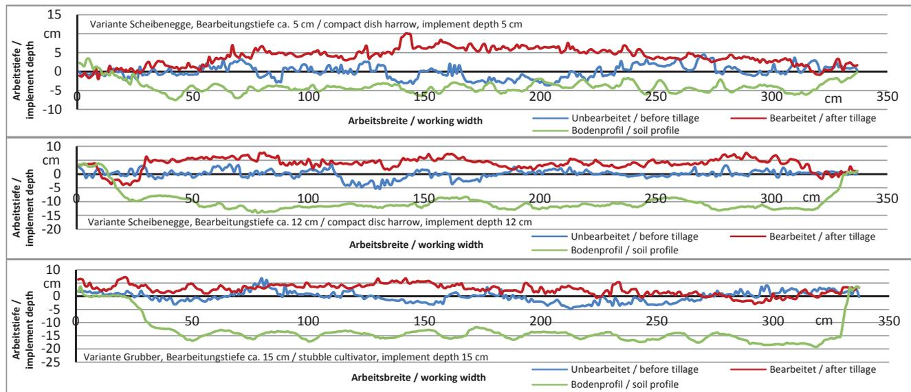
Typical soil profile of compact disc harrow and stubble cultivator before and after tillage
