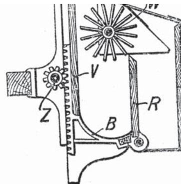
With the 1885 Schloer fertiliser spreader, the hoppers were moved to the spreading mechanism via rack and pinion gearing
