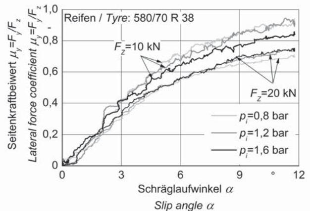
Quasi steady-state lateral force coefficient at different stationary loads and tyre pressures for a 580/70 R 38 tyre on asphalt
