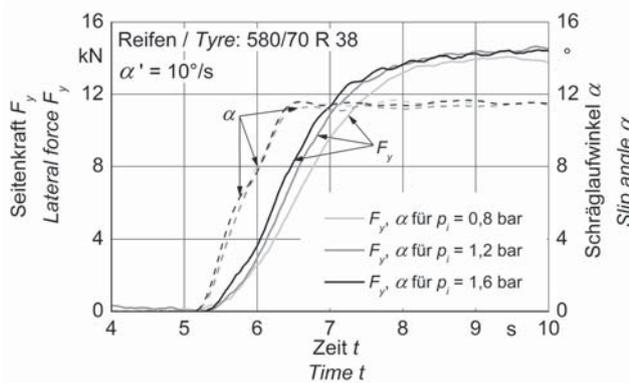
Measured slip angle and the corresponding lateral forces for a 580/70 R 38 tyre at different tyre pressures and a stationary wheel load of 20 kN
