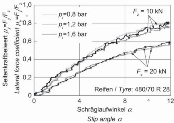
Quasi steady-state lateral force coefficient at different stationary loads and tyre pressures for a 480/70 R 28 tyre on asphalt
