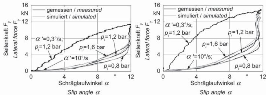
Measured and simulated lateral forces on a 480/70 R 28 tyre (left) and a 580/70 R 38 tyre (right) under different tyre pressures, slip angle rates (0,3°/s and 10°/s) and a constant vertical load of 20 kN on asphalt
