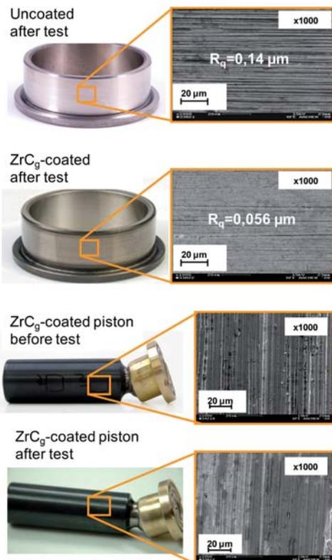
Rolling bearings after test (top), pistons before and after test (bottom)
