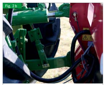
Clearance between tractor and fertilizer spreader
