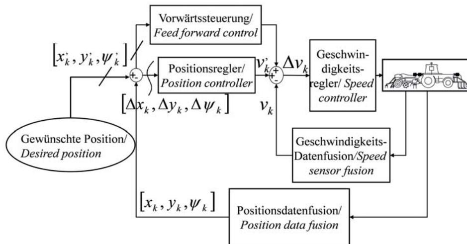
Structure of the cascade controller with feed forward control for the speed regulation
