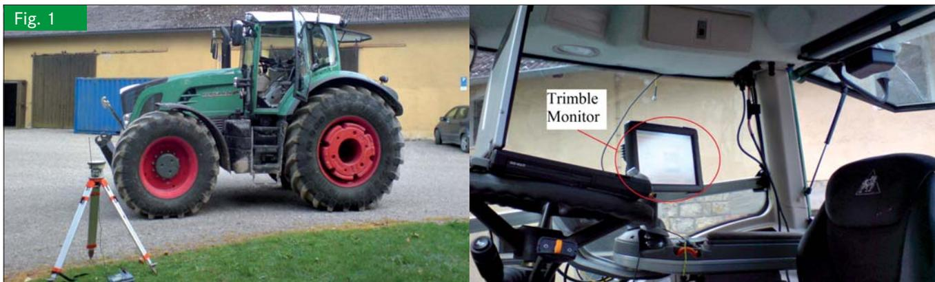
Fig. 1 Fendt 936 Vario tractor and its cabine with navigation monitor from Trimble
