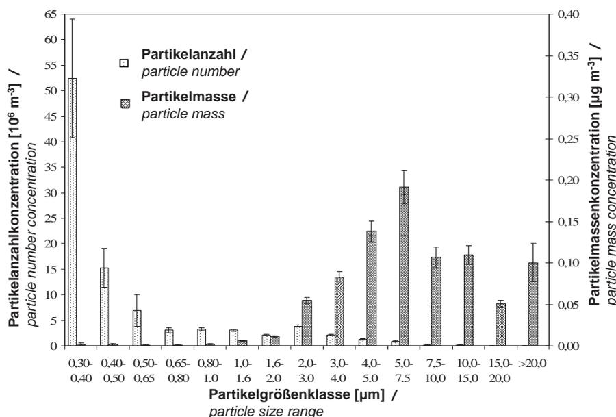
Particle number- and particle mass distribution in the outlet air of a deep litter system [9]
