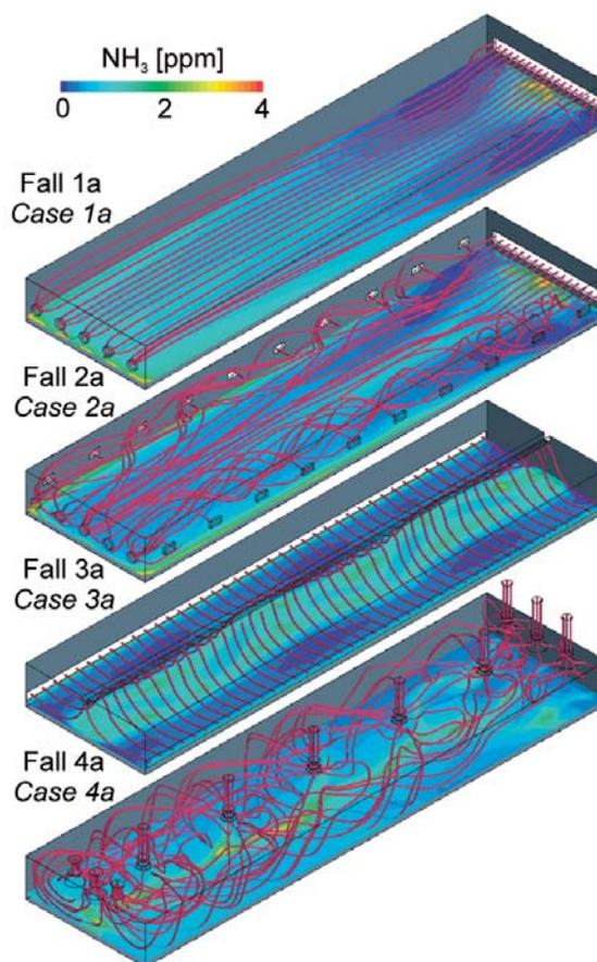
The ammonia concentration distribution at 0.5 m is shown for the first four cases in the free poultry stable areas. The concentration at the bottom is in all cases 20 ppm.
