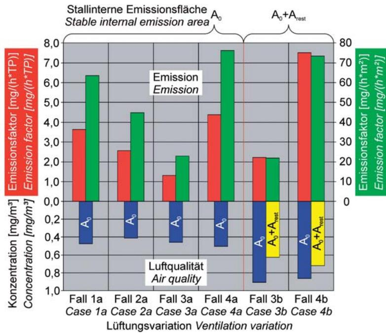
In dependency on the arrangements (1a to 4a without aviary frames and 3b to 4b with aviary frames) the emission factors are shown in the upper part with regard to the animal (red) resp. with regard to the emission area (green) and in the part below the mean concentration 0.2 m above the internal emission areas of the stable. The stables with lowest emissions are those ones with line sources and sinks
