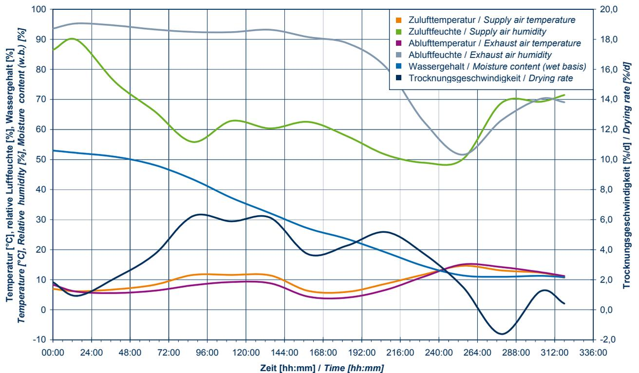
Fig. 3: Drying process of wood chips (poplar, chunky pieces)
