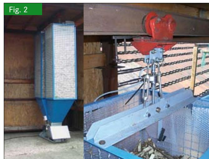
*Fig. 2: Sample container for drying of wood chips (left), registration of weight loss by a load cell (right)*
