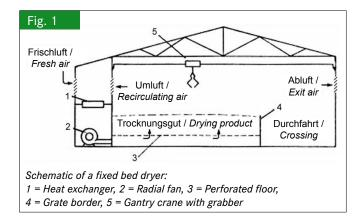
purpose drying method are the comparatively simple structure of the dryer, the immediate drying without interim storage, and the relatively low labour demand. As yet, a main disadvantage is the high specific energy demand (up to one liter of fuel oil, or an equivalent effective amount of natural gas per kg of dried material) due to uneven air flow distribution, inhomogeneous bed material distribution on the drying grates, insufficient air circulation and high heat loss [2].
