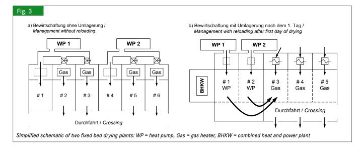
in which about two thirds of utilized primary energy is wasted, the waste heat of a combined heat and power plant can be used to reduce fuel consumption in the conventional drying phase. Moreover, the comparatively dry and warm exhaust air from the conventional drying area can be utilized as inlet air for another drying hall (not depicted).
