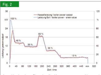
Annual load cycle profile and realized heat power output with a wood chip boiler
