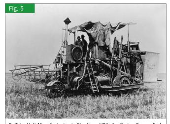
Built by Holt Manufacturing in Stockton, USA: the first self-propelled combine harvester powered by a petrol engine
