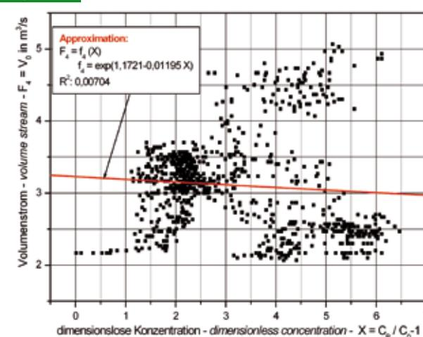
Volumetric flow rate versus the dimensionless concentration X. F<sub>4</sub> determines the approximation function
