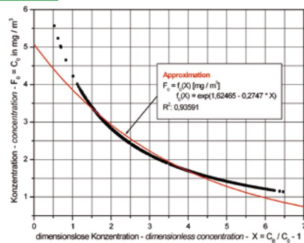
Ammonia concentration versus the dimensionless concentration X. F<sub>0</sub> determines the approximation function
