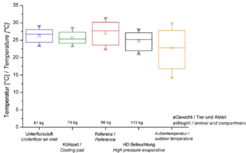
Range of temperatures of inlet air and indoor air
