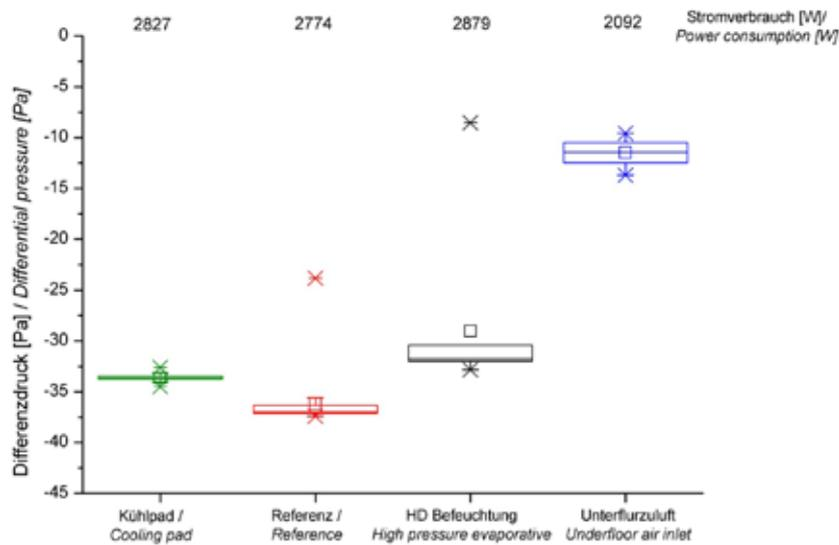
Differential room pressure at fan capacity of 100 % during four hours
