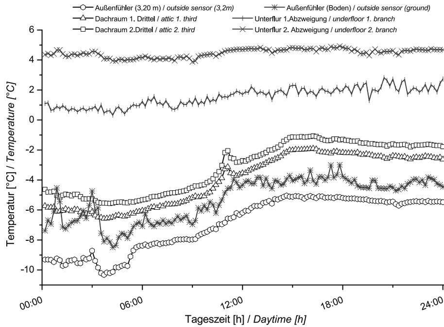
Difference in temperature rise between air supply via attic or underfloor
