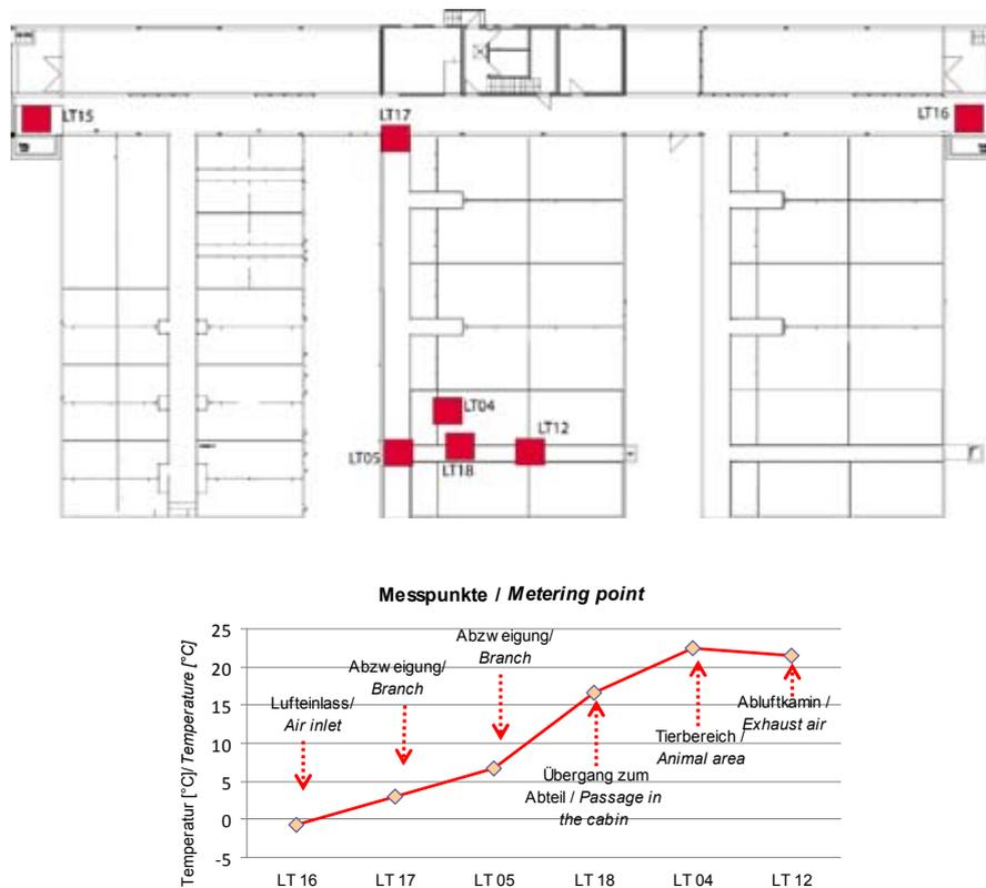
Position of the temperature sensors and course of temperature at a cold day using the example of the variant underfloor air inlet
