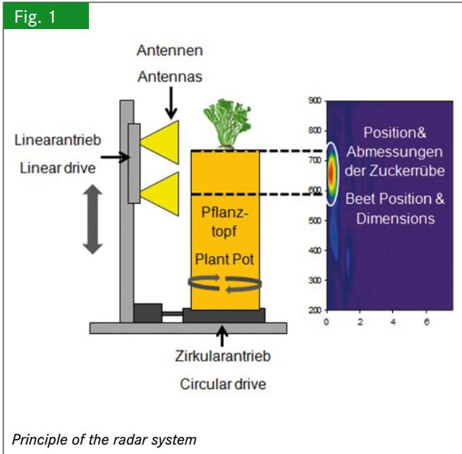
ear drive) and positioning of the plant pot in horizontal direction (circular drive). The reflected part of the electromagnetic waves was recorded by the RADAR-system at each position of the scanner. Further data processing was done using the software Matlab. The principle of the whole system is illustrated in **Figure 1**.
