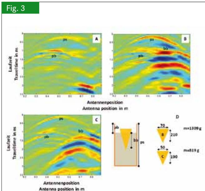
*Radargrams of reference measurement (A) and measurement of different topped sugar beets (B and C) in quartz sand (volumetric moisture 9.6 %). Distinctive reflection characteristics are marked in the radargrams. The marks, the dimensions of the different sugar beets (in mm) and their mass are explained in D): ps: plant pot surface, pb: backside of the plant pot which is not covered by quartz sand, bb: beet body*
