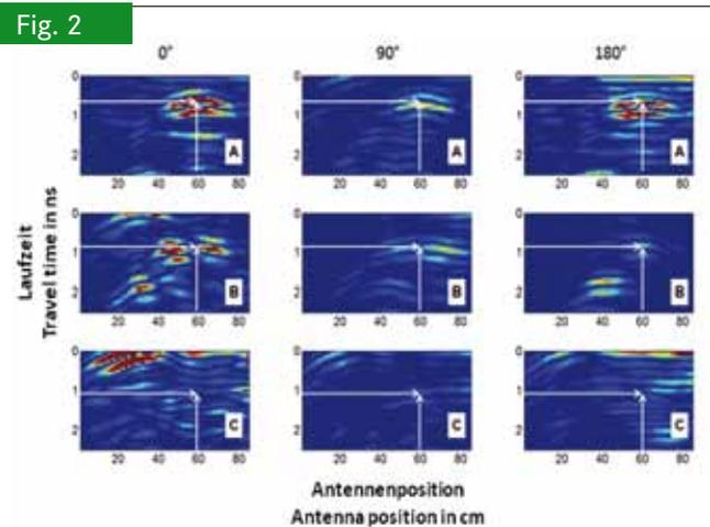
*B-Scans (radargrams) of water saturated 120 mm test-body from different shooting angles. The volumetric moisture of the quartz sand was 7.2 % (A), 12.4 % (B) and 22.4 % (C). The white arrows indicate the approximate position of the test body in time-domain and on the scanner track.*
