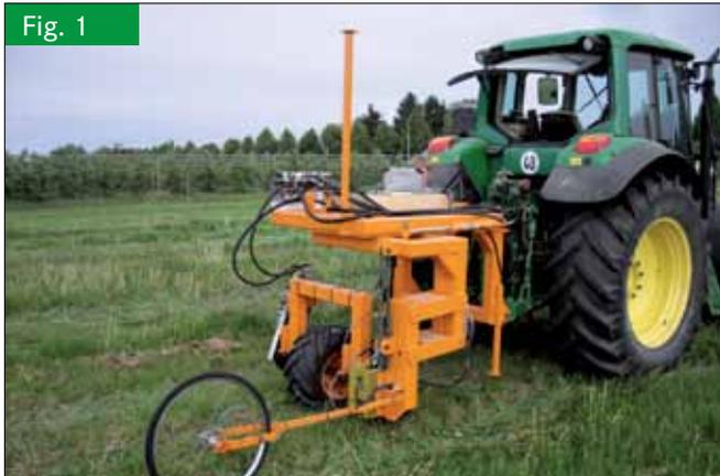
Test rig for single wheels on test run with small tractor tire
