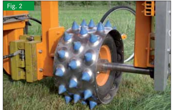
Studded roller-wheel in test rig for single wheels on grass stubble
