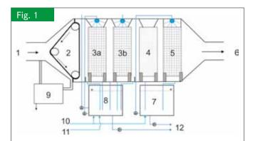
Test facility 1 for poultry exhaust air cleaning (1: raw gas, 2: dust filter with reclaimable filter pad, 3a: scrubbing unit 1, 3b: scrubbing unit 2, 4: odor reduction unit, 5: scrubbing unit 3, 6: clean gas, 7: reservoir 2, 8: reservoir 1, 9: dust exhaustion and removal, 10: fresh water supply, 11: sulfuric acid supply, 12: waste water discharge)
