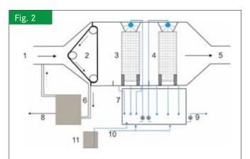
Test facility 2 for poultry exhaust air cleaning (1: raw gas, 2: dust filter with reclaimable filter pad, 3: scrubbing unit 1, 4: scrubbing unit 2, 5: clean gas, 6: filter pad exhaustion, 7: reservoir, 8: dust removal, 9: waste water discharge, 10: fresh water supply, 11: sulfuric acid supply)
