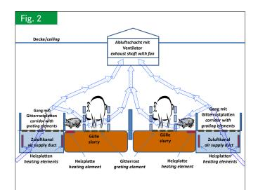
Air flow from underfloor area into the compartment
