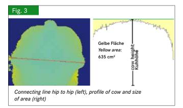
and a list is generated with characteristics, cow-ID and date. Depending on cow-ID and timestamp the parameters can be connected with management data.
