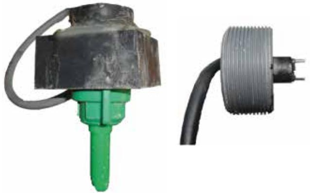
Sensor for in-tube and nozzle holder measurement (Photo: J. Geiß)
