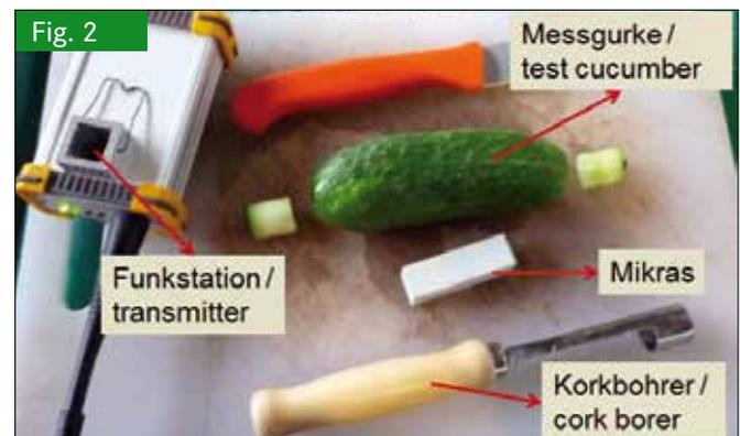
Implantation of the 3D-acceleration sensor Mikras into a test pickling cucumber (Foto: J. Surdilovic)
