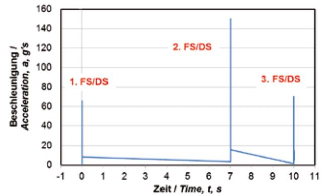
Example of measured impact acceleration with an implanted test pickling cucumber over one cycle from intake unit to sorting conveyor (DS 1-4, Fig. 1)
