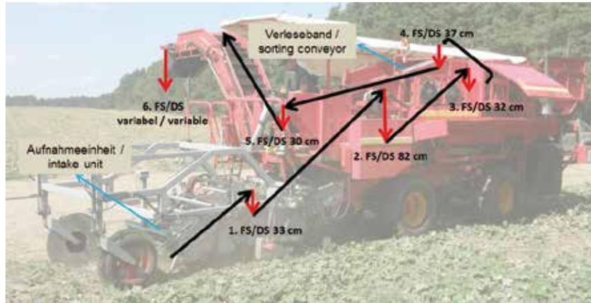
Drop steps (DS) of the fully mechanized harvesting machine Pomac (Foto: M. Geyer)
