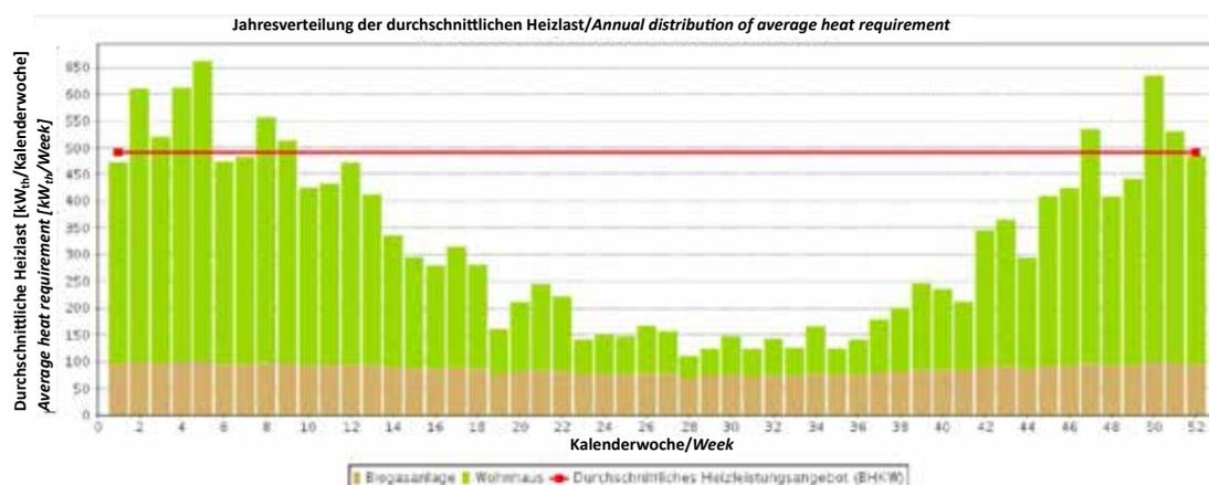
Annual distribution of average heat requirement of 500 kW<sub>el</sub> biogas plant incl. 80 single-family houses (built 1978 to 1995) and idealised heat supply from a biogas plant (red line)
