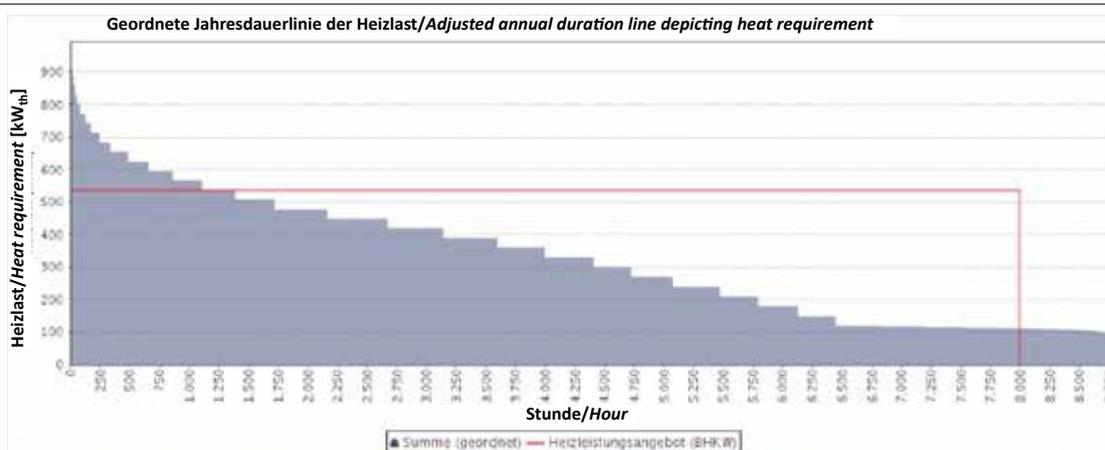
Adjusted annual duration line depicting heat requirement of a 500 kW<sub>el</sub> biogas plant incl. 80 single-family houses (built 1978 to 1995) and idealised annual duration line of heat supply of a biogas plant (red line); peak load: heat total 123,042 kWh<sub>th</sub> per annum.
