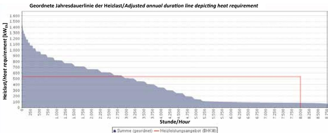
Adjusted annual duration of heat requirement from a 500 kW<sub>el</sub> biogas plant incl. 10,000 m<sup>2</sup> greenhouse and idealised annual duration line of the heat production of biogas plant (red line); peak load: heating performance 1,062 kW<sub>th</sub>, heat total 745,325 kWh<sub>th</sub> per annum.
