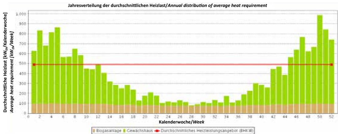
Annual distribution of average heat required from a 500 kW<sub>el</sub> biogas plant incl. 10,000 m<sup>2</sup> greenhouse and idealised heat production of biogas plant (red line)
