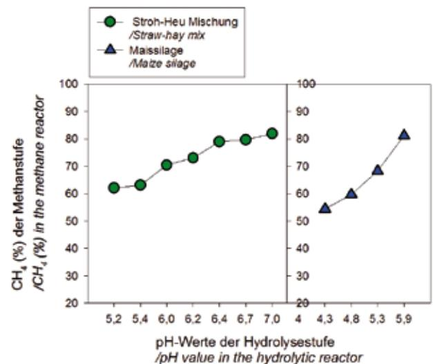
Methane content in the methane digester for the straw-hay mix and for maize silage
