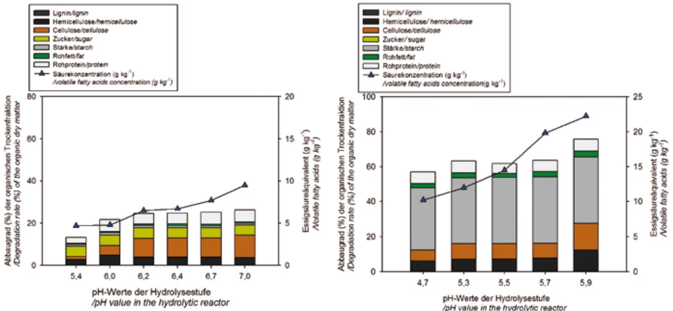
Degradation of the substrate in the hydrolytic reactor of a two stage system, straw-hay mix (left), maize silage (right)
