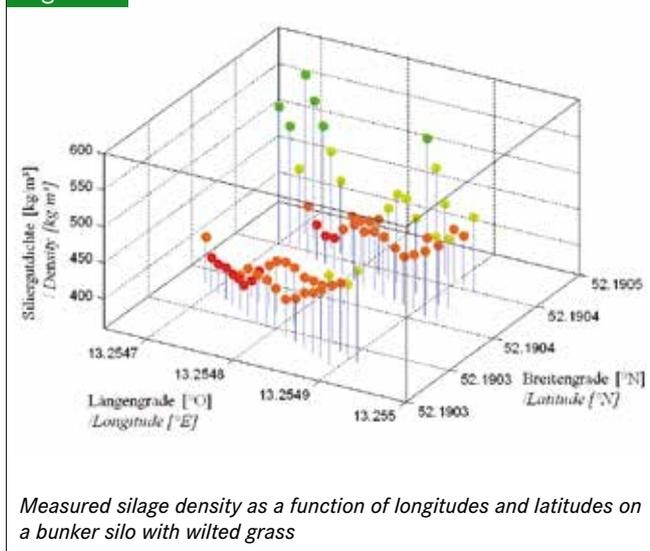
By means of own preliminary tests regarding the penetration depth of the gamma rays it is known, that density differences inside the material at 760 kg/m<sup>3</sup> (dry mass) can be observed up to a depth of 10 cm [5]. This implies for the compaction drives that the density value determined is representative for the upper material layer, which is just compacted.
