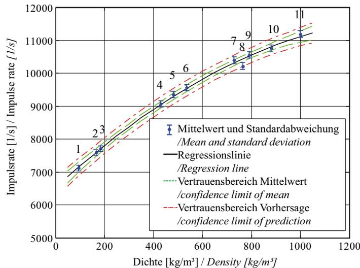
Calibration curve with confidence areas for the radiometric density measuring device: 1 balsa, low density, 2 hemp shives, 3 balsa, high density, 4 spruce, natural, 5 oats, loosely poured, 6 oats, firmly tapped, 7 rye, loosely poured, 8 oak, 9 rye, firmly tapped, 10 spruce, compressed, 11 water
