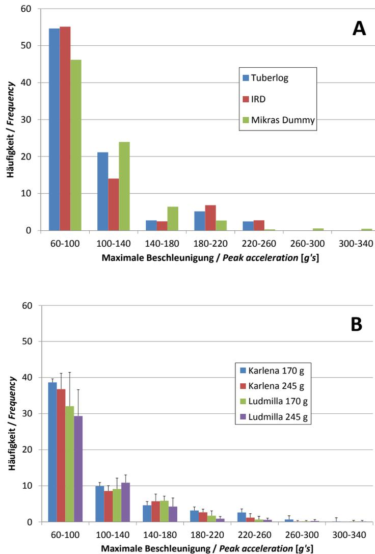
Frequency distribution of impacts with peak acceleration of  $\geq 60$  g/s measured with electronic fruits (A) and Mikras in potato tubers (B) during 10 runs through a processing line simulator (conveyor speed  $0.35 \text{ m s}^{-1}$ )
