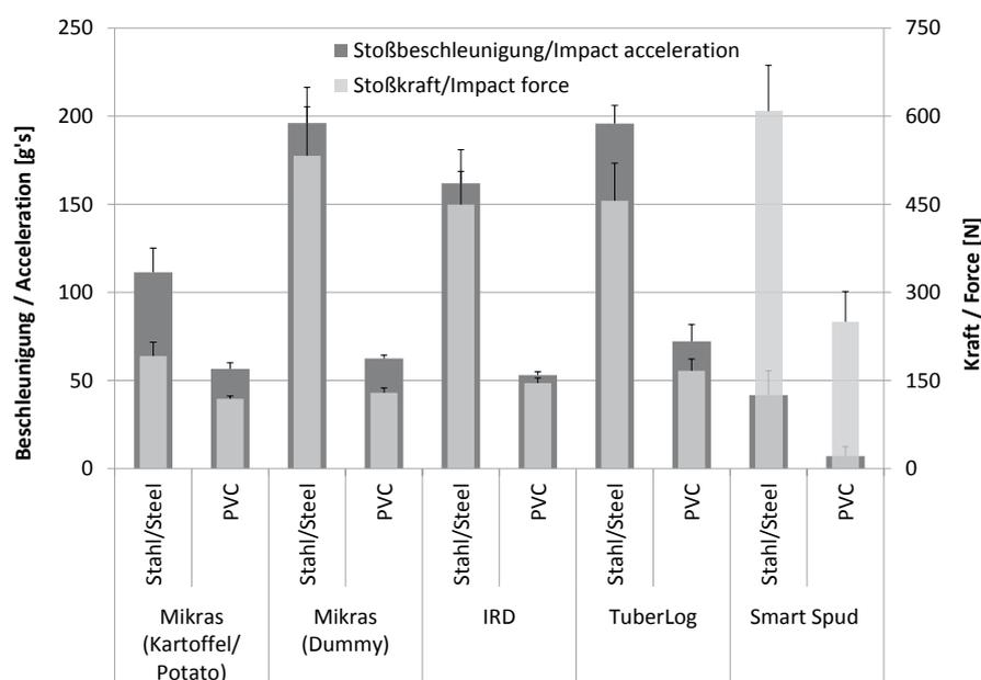
Peak acceleration measured from different electronic fruits (lateral drop, height 10 cm, onto steel or PVC) and peak force measured by a sensor in the drop simulator
