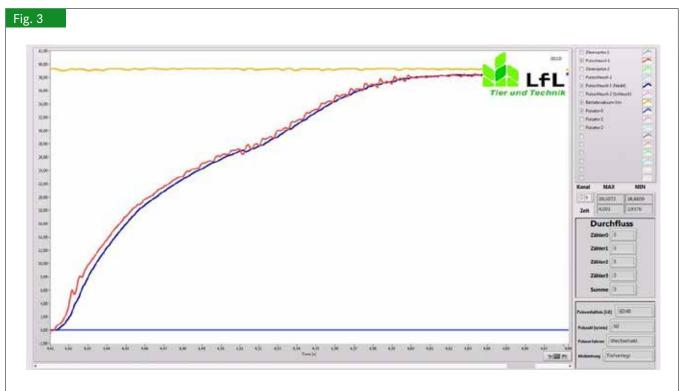
Results of an example measurement (yellow - operating vacuum; red - measuring point within the short pulse tube; blue - measurement with needle and tube (inside diameter Ø 4 mm, 30 cm long))
