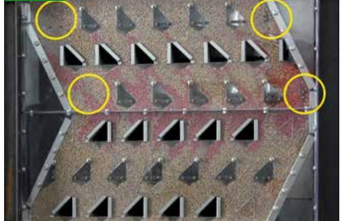
Particle flow profile in the new designed dryer geometry with optimized number of air ducts (Photo: ATB)
