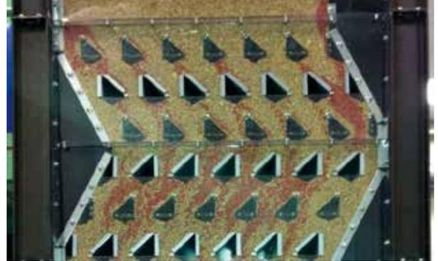
Particle flow profile of colored wheat particles in the test dryer with new design and maximum number of air ducts (Photo: ATB)
